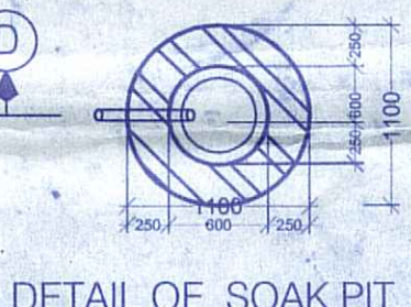
DETAIL OF SOAK PIT SCALE:1:50
